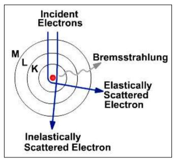
The electron may get deflected from 0- $90^{\circ}$ ; if it gets a deflection of  $90^{\circ}$  (the probability of which is very small), almost all of its kinetic energy is lost and x-ray photon of high energy (equivalent to the kinetic energy of the incoming electron) will be formed. It means that an electron may loose all, none or an intermediate level of its kinetic energy in Bremsstrahlung interaction. Therefore xray produced will be of heterogeneous/
